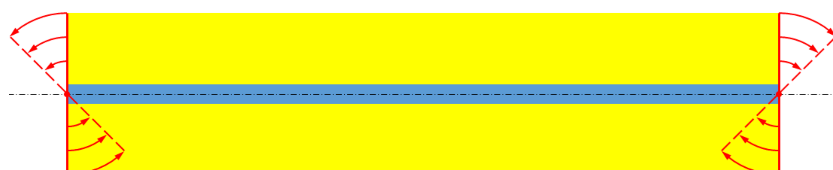
Figure 2: Cross section view of the flexible foil with one layer of AlCu interconnects. Rotational displacements of the edges in a circular way around the neutral axis (black dotted line) are highlighted in red.
