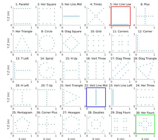
Fig. 3: 2D sensor configurations for 16 sensors. Configurations were applied horizontally (at  $z:0$ ) and vertically (at  $y:0$ ). The Cramér-Rao lower bound analysis indicates that *30:HorFours* (green) and *22:VertLineMid* (blue) performed best horizontally and vertically, respectively. *5:HorLineLow* (red) is indicated as the worst performing configuration.
