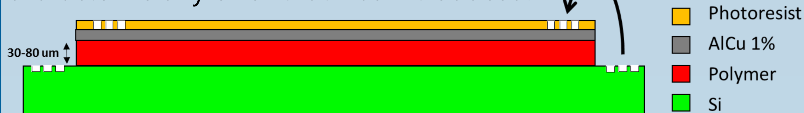
Figure 5. Cross-section showing the layers fabricated to create a geometric simulation of the proposed 'terraced' wafer.
